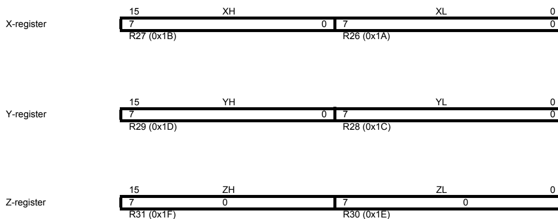
Figure 4-3. The X-, Y-, and Z-registers
