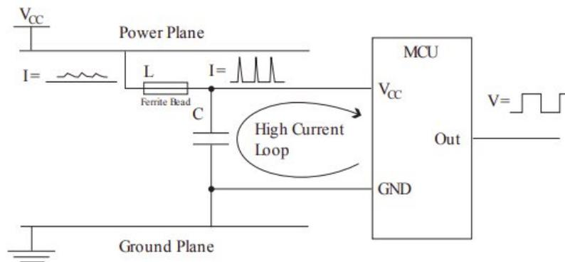
In Atmel AVR devices where power and ground lines are placed close together there will be better decoupling than the devices with industry standard pin-out. In industry standard pin-out, the power and ground pins are placed in opposite corners of the DIP package. This disadvantage can be overcome by placing decoupling capacitors very close to the die. For devices with multiple pairs of power and ground pins, it is essential that there is a decoupling capacitor for every pair of pins.
